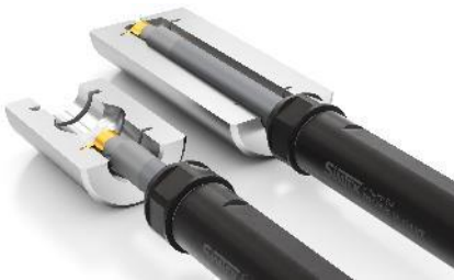
Figure 3: simturn DX Caption: simturn DX toolholders with steel round shank for the internal machining of small components can be used in variable lengths. Thanks to the friction-locked ME - clamping system, the internal carbide toolholder is clamped securely.
